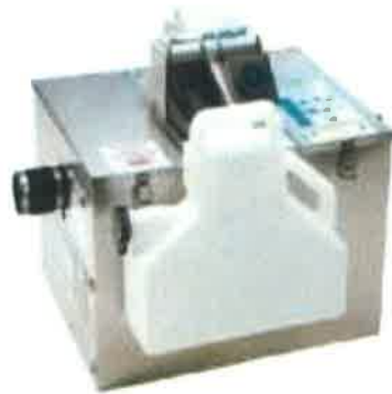
Automatic Grease-Recovery Unit (AGRU)
